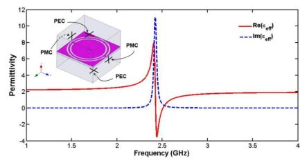
Figure 3. Simulation model and retrieved effective permittivity of the CSRR unit cell.
