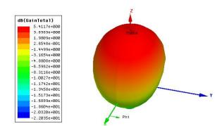
Figure 8. 3D gain pattern of the MIMO antenna while excited only port 1.
