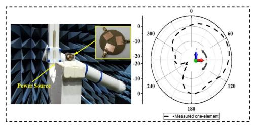
*Figure 10.* Radiation pattern and gain measurement of the proposed MIMO antenna. The fabricated antenna is depicted in the pattern chamber.
