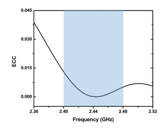
Figure 6. ECC of the proposed MIMO antenna.
