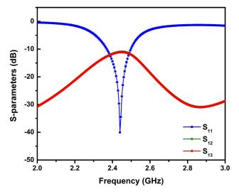
Figure 4. S-parameters of the proposed MIMO antenna.
