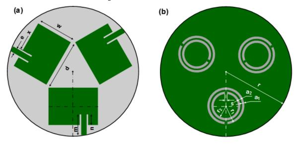
*Figure 1.* Geometry of the proposed three-port metamaterial MIMO antenna: (a) top view and (b) bottom view.
