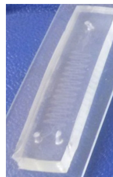
Fig. 3. An image of a PDMS-based microfluidic device (observed under the camera of an iPhone 5).
