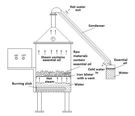
Fig. 1. Diagram of steam distillation system.
