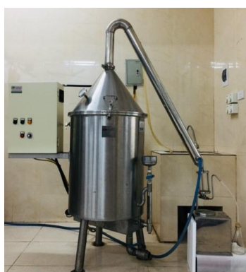
Figure 3. Steam distillation equipment at the laboratory of Vinh University
