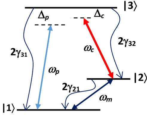
**Figure 1.** The excitation scheme of the closed-loop three-level lambda-type system.
