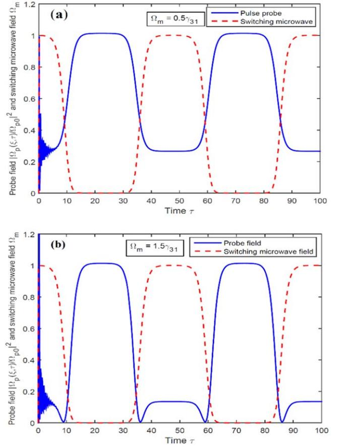
**Figure 7.** Time evolution of the probe field (solid line) at  $\xi = 50/\alpha$  for different intensities of the microwave field:  $\Omega_{m0} = 0.5\gamma_{31}$ ; (b)  $\Omega_{m0} = 1.5\gamma_{31}$ . The other parameters are  $\phi = \pi/2$ ,  $\Omega_c = 10\gamma_{31}$ ,  $\Omega_p = 0.5\gamma_{31}$ ,  $\Delta_p = 0$ ,  $\Delta_c = 0$ ,  $\gamma_{32} = \gamma_{31}$ , and  $\gamma_{21} = 0$ .
