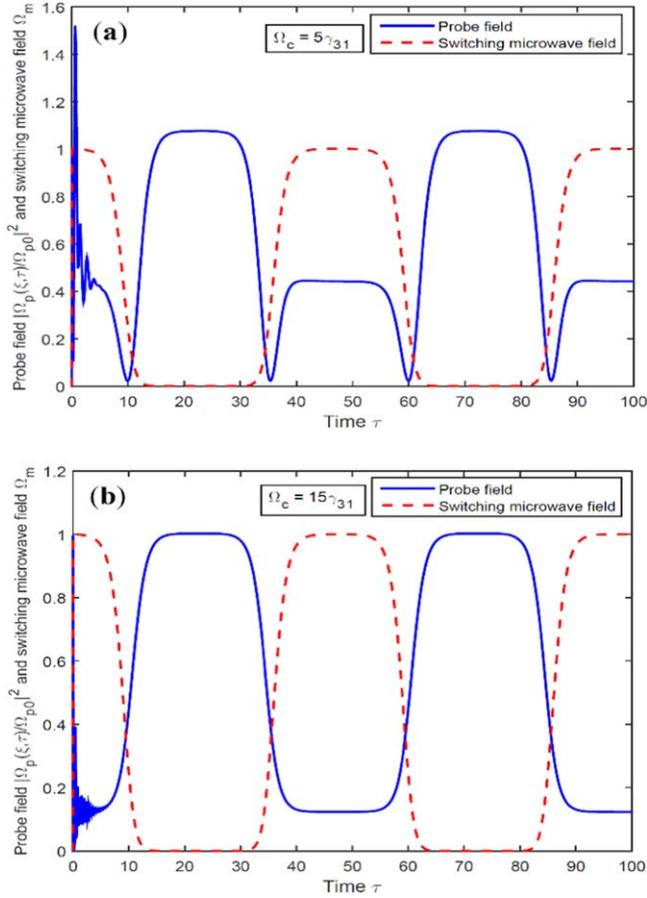
**Figure 6.** Temporal evolution of the probe field (solid line) at  $\xi = 50/\alpha$  for  $\Omega_c = 5\gamma_{31}$  (a) and  $\Omega_c = 15\gamma_{31}$  (b). Other parameters are  $\phi = \pi/2$ ,  $\Omega_p = 0.5\gamma_{31}$ ,  $\Omega_{m0} = \gamma_{31}$ ,  $\Delta_p = 0$ ,  $\Delta_c = 0$ ,  $\gamma_{32} = \gamma_{31}$ , and  $\gamma_{21} = 0$ .
