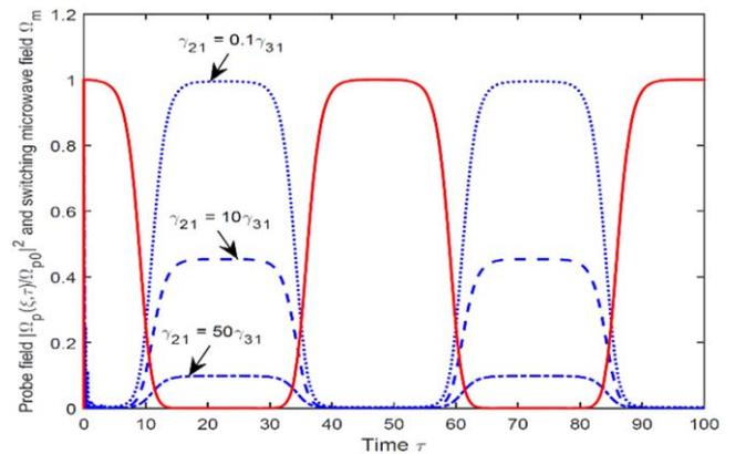
**Figure 8.** Variation of the transmitted probe field at  $\xi = 50/\alpha$  for different decay rates:  $\gamma_{21} = 0.1\gamma_{31}$  (dotted line),  $\gamma_{21} = 10\gamma_{31}$  (dashed line), and  $\gamma_{21} = 50\gamma_{31}$  (dot-dashed line), when the microwave field (solid line) is switched at the period  $50/\gamma_{31}$ . The remaining parameters are the same as in figure 5.
