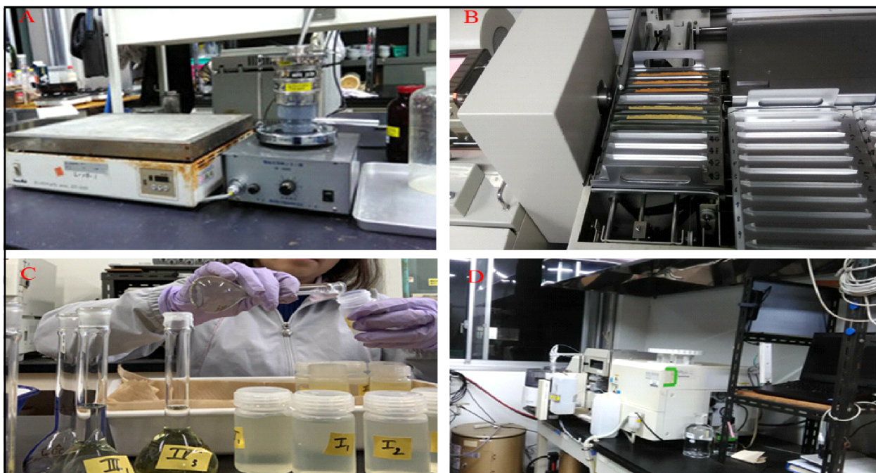
Fig. 4. Illustrations of types of equipment for investigating PFOS a) equipment for sieving and heating samples EC-1200, b) equipment for soil sample analyses N-C coder, c) prepare samples and d) analysis atomic absorption spectrophotometer (AA-6800).
