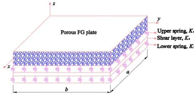
Fig. 1. The configuration of rectangular FGP plates resting on the Kerr foundation.
