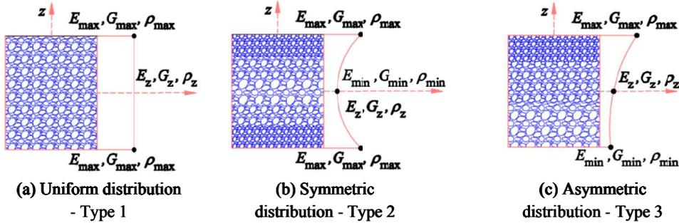
Fig. 2. The FGP plate with different porosity density distribution patterns.
