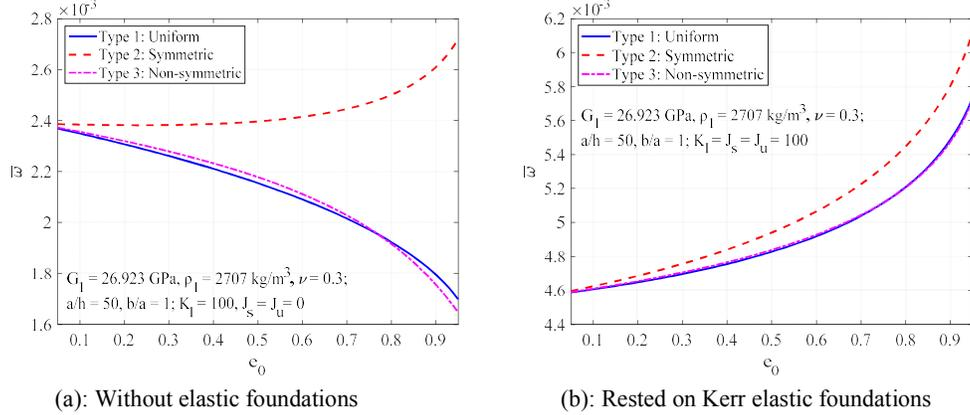
**Fig. 2.** Variation of the non-dimensional natural frequency of FGP plate with porosity coefficients  $e_0$  and various porosity distribution patterns.
