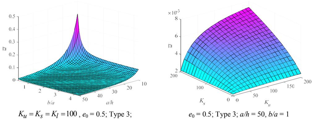
**Fig. 3.** Variation of non-dimensional natural frequency of the FGP plate versus  $b/a$  and  $a/h$  ratios.
