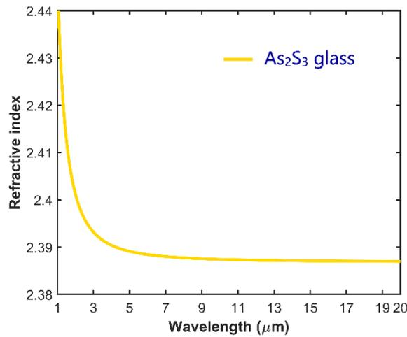
Fig. 1. Refractive index  $n$  of the chalcogenide glass  $\text{As}_2\text{S}_3$  as a function of the wavelength  $\lambda$ .
