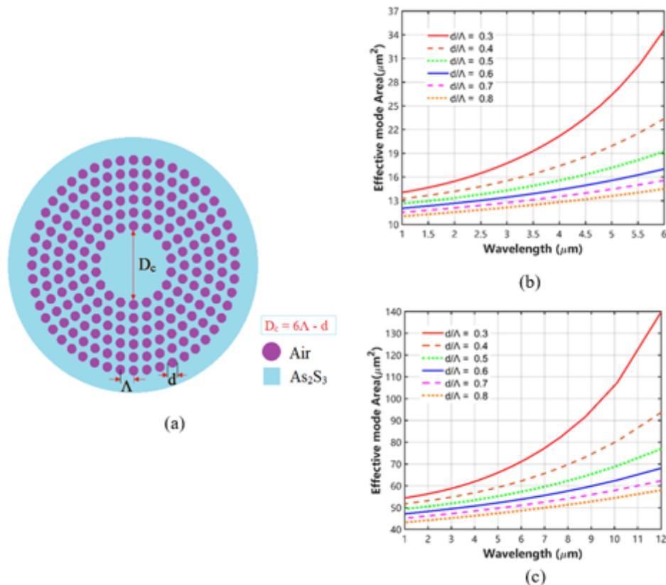
Fig. 2. For the  $\text{As}_2\text{S}_3$  PCF,  $D_c = 6\Lambda - d$ . Structural diagram of PCFs (a), effective mode area  $A_{\text{eff}}$  of PCFs as a function of wavelength at a hole-pitch of 1  $\mu\text{m}$  (b) and 2  $\mu\text{m}$  (c).
