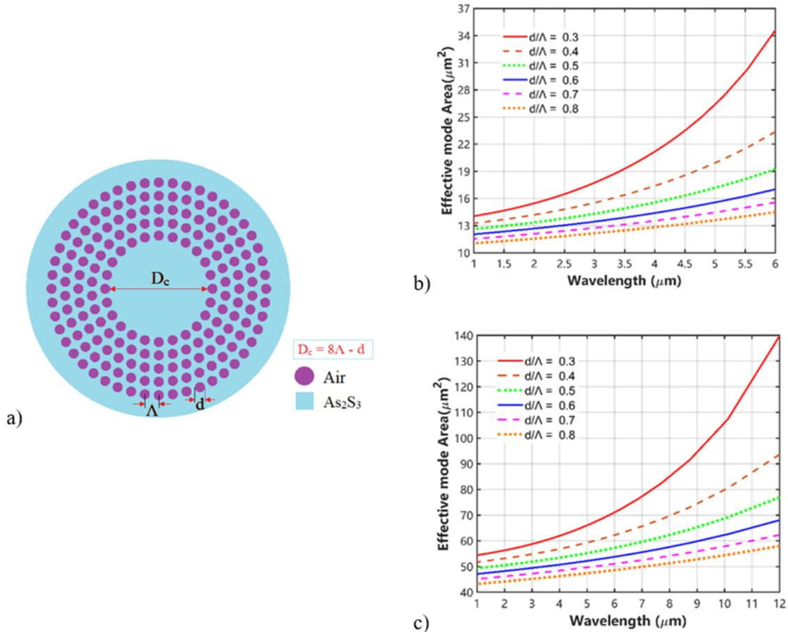
**Fig. 3.** For the As<sub>2</sub>S<sub>3</sub> PCF,  $D_c = 6\Lambda - d$ . Structural diagram of PCFs (a), effective mode area  $A_{eff}$  of PCFs as a function of wavelength at a hole-pitch of 1  $\mu\text{m}$  (b) and 2  $\mu\text{m}$  (c).
