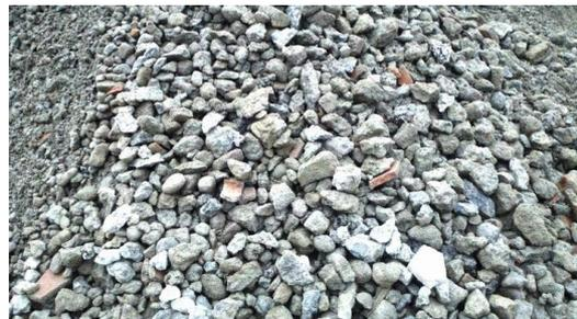
Fig. 1. Recycled coarse aggregates
