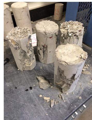
Fig. 3. Samples after the compressive experiments.
