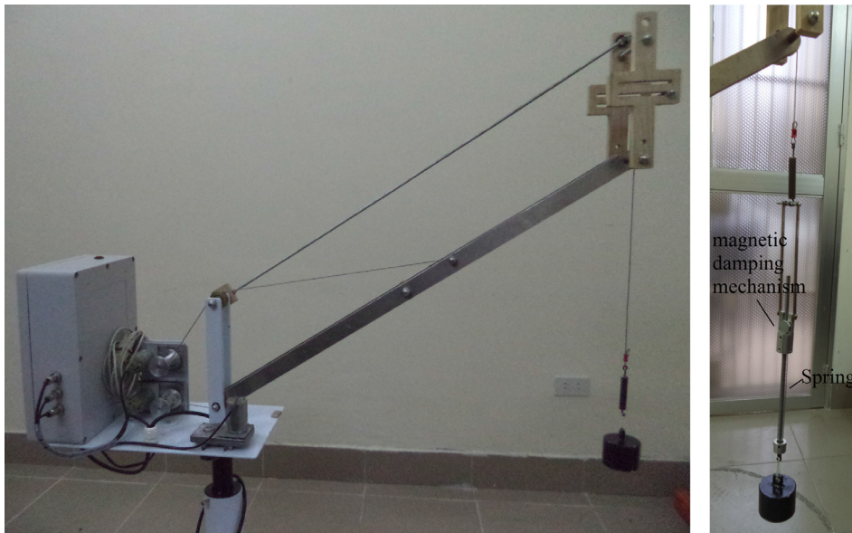
Fig. 11. Boom crane (a) and spring-damper mechanism (b).
