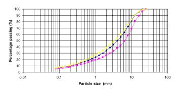
Fig-3: Particle size distribution by sieving
