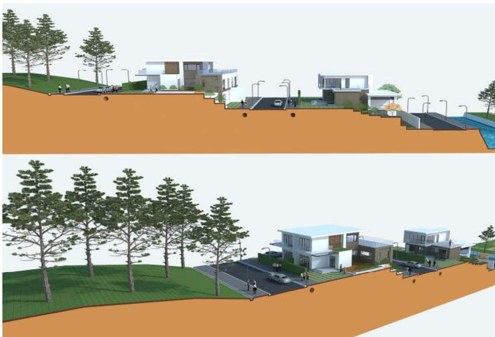
Fig. 6. Proposed cross-section of architectural space of residential area.
