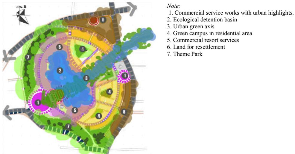
Fig. 5. The proposal for floor-plan of functional zoning.
