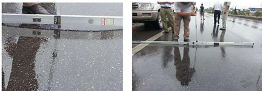
**Fig. 2.** Depth measurement of ruts at National Highway 1 section Vinh-Ha Tinh [1].
